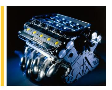
The RS2 engine slotted even more seamlessly into Williams' FW13B chassis, courtesy of its smaller size (4.8cm shorter and 1.5cm lower). It was also 2kg lighter than before, with timing gears replacing the former timing belts. Notwithstanding these improvements, it was a difficult season for Patrese and Boutsen as rivals Ferrari and Benetton-Ford leapfrogged Williams-Renault into second and third respectively behind the still dominant McLaren-Honda.
